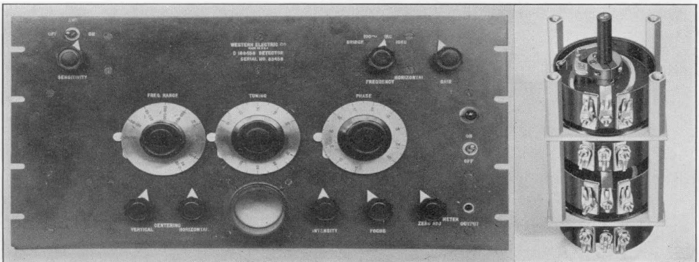
Figure 14. Panel view (left) of a Western Electric detector used in checking coils. The four-gang rheostat controlled by the TUNING dial is shown at the right.
