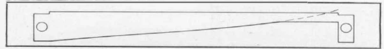
Figure 15. Mandrel shape used for the "C"-bias rheostat in the tube checker of Figure 16.
