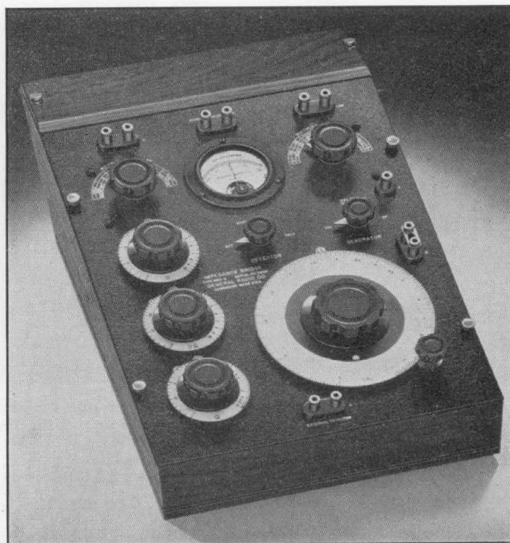
Figure 11. Panel view of the Type 650-A Impedance Bridge. The logarithmic rheostat controlled by the large dial was shown in Figure 2, Part I, of this article.
